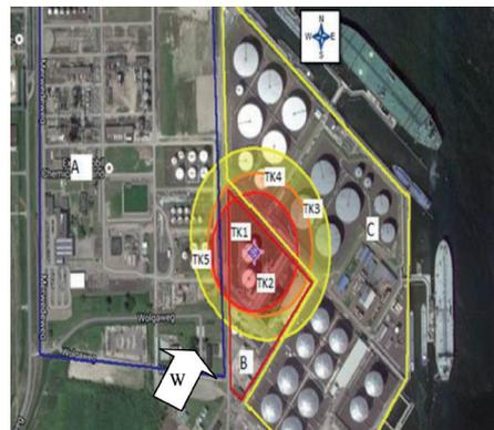
Figure 4. Pool fire at TK1, footprint-effected zones calculated by ALOHA.
